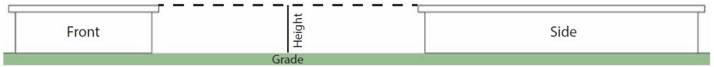
Figure 1 - Diagram showing how to measure height for flat roof construction.
