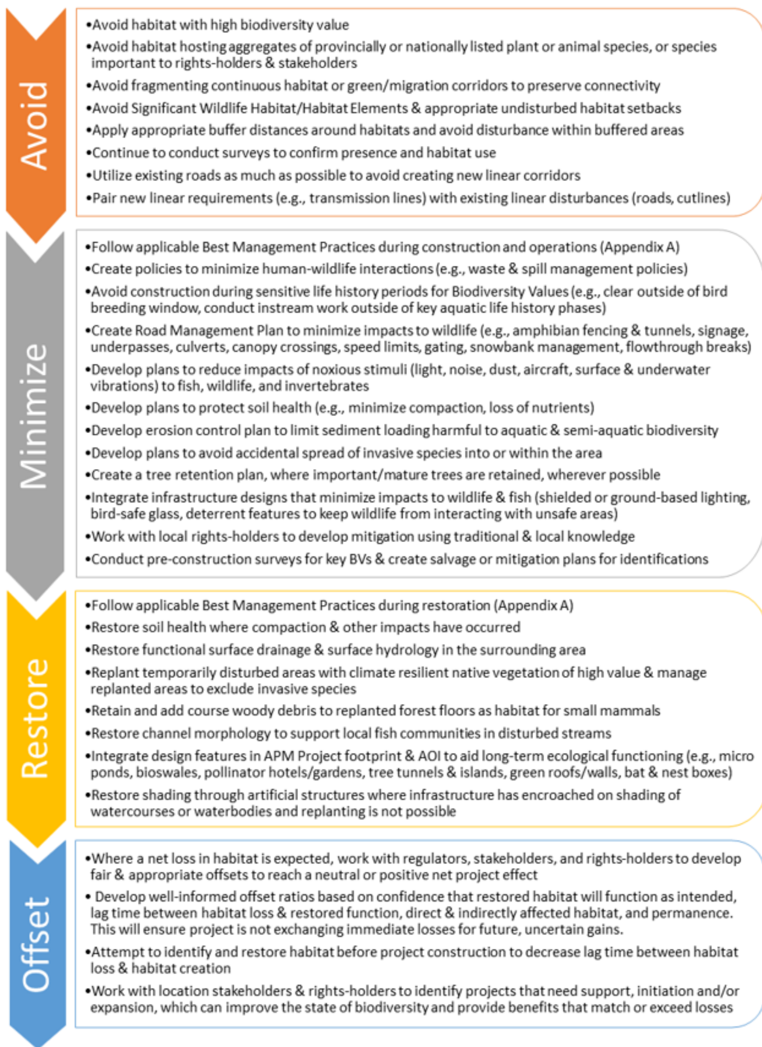
Figure 4-1. Steps of the mitigation hierarchy including avoidance, minimization, restoration, and offset options to eliminate or reduce the magnitude of impacts at each step. While the last stage in the mitigation hierarchy is acknowledged to be “offset”, offset will only be considered after other steps along the mitigation hierarchy are applied to their maximum feasible extent, and a residual effect remains.
